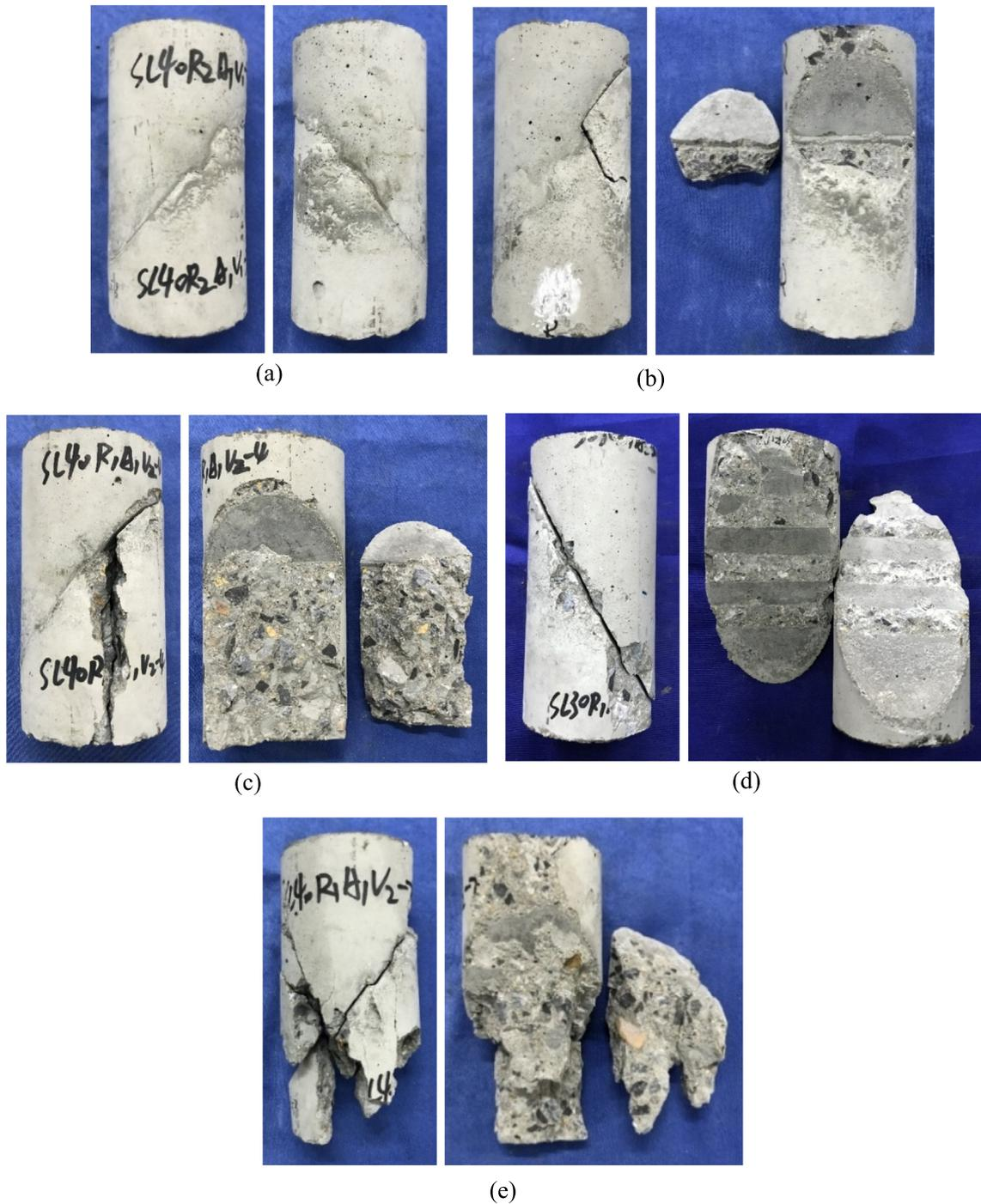
**Fig. 5.** Typical failure modes of slant shear specimens: (a) M1 (SL40R2A1V1); (b) M2 (SL30R2A1V1); (c) M3 (SL40R1A1V2); (d) M4 (SL30R1A2S); and (e) M5 (SL40R1A1V3).
